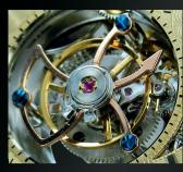
Breguet from an earlier idea by the English chronometer maker John Arnold, a tourbillon aims to counter the effects of gravity by mounting the escapement and balance wheel in a rotating cage, to negate the effect of gravity when the timepiece (and thus the escapement) is stuck in a certain position.
