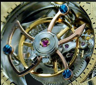
Breguet from an earlier idea by the English chronometer maker John Arnold, a tourbillon aims to counter the effects of gravity by mounting the escapement and balance wheel in a rotating cage, to negate the effect of gravity when the timepiece (and thus the escapement) is stuck in a certain position.
